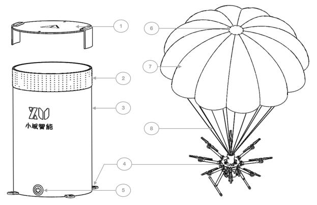
①: cover ②: magic post ③: parachute barrel ④: fixing hole ⑤: switch ⑥: air hole ⑦: canopy ⑧: cord
